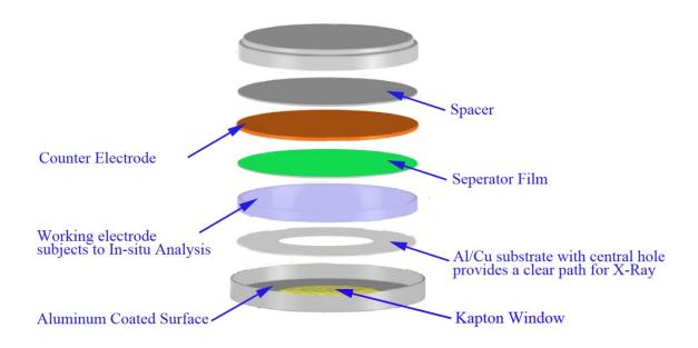
Since the internal space of the coin cell is 16.5mm I.D x 1mm H., the recommended height of the stacking materials is at least 1mm. This will ensure a solid metal contact inside the cell. Here we illustrate the preparing methods of the stacking materials:
